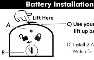
D) Install 2 AA batteries (must be new). Watch for polarity
